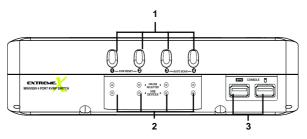
**KVM Status LEDs:** Lights DIM ORANGE to indicate that the computer attached to the corresponding port is up and running (On Line); lights BRIGHT ORANGE to indicate that the computer attached to its corresponding port is the one that has the KVM focus (Selected); flashes to indicate that the computer attached to its corresponding port is being accessed under Auto Scan mode.
